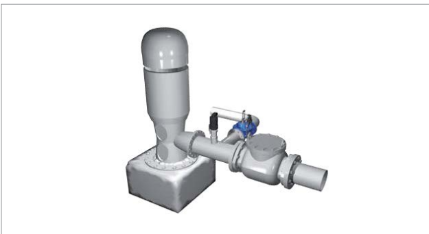
FIG. 8 Discharge side of vertical turbine pumps
