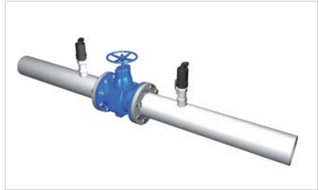
FIG. 10 Both sides of check-valves, isolating valves and any device that may be closed
