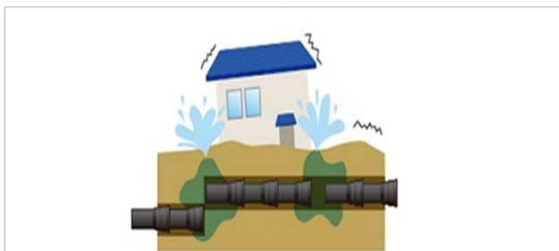
FIG. 1 Example of joint separation.
